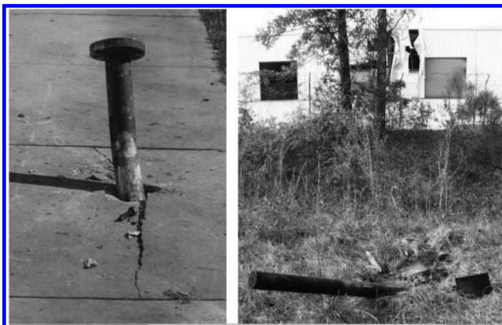
Figure 11. Portions of T2 reactor piping and agitator shaft embedded in surrounding areas caused by T2 explosion. Photographs courtesy of U.S. Chemical Safety and Hazard Investigation Board, taken from Investigation Report No. 2008-3-I-FL, September 2009
