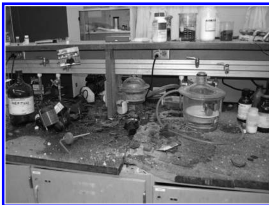
Figure 27. Aftermath of Texas Tech lab explosion. Photograph courtesy of U.S. CHEMICAL SAFETY AND HAZARD INVESTIGATION BOARD, taken from CSB Case Study NO. 2010-05-I-TX (38)
