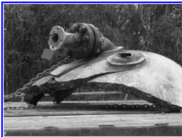
Figure 10. Portion of the 3 inch thick steel reactor wall after T2 reactor explosion. Photograph courtesy of U.S. Chemical Safety and Hazard Investigation Board, taken from Investigation Report No. 2008-3-I-FL, September 2009
