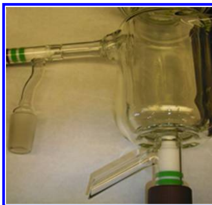
Figure 10. A standard 100 mL lab reactor retrofitted by adding an overflow valve to allow continuous operation.
