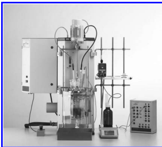
Figure 13. Mettler-Toledo RCI calorimeter. Photo used with permission of Mettler-Toledo AutoChem, Inc.- www.mt.com/autochem
