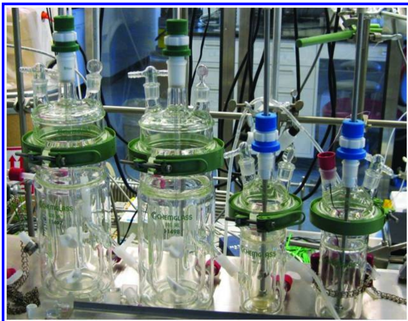
Figure 10. Photo of CSTR rig set up with a train of 2 x 800 mL and 2 x 100 mL reactor vessels.
